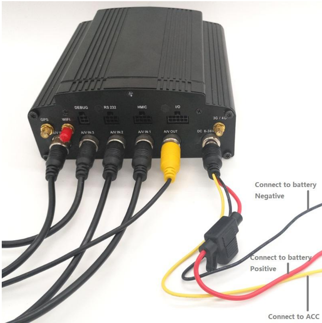
2: MDVR connection with UPS:
